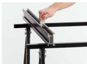
Prepare the sub-construction frame with corner piece
